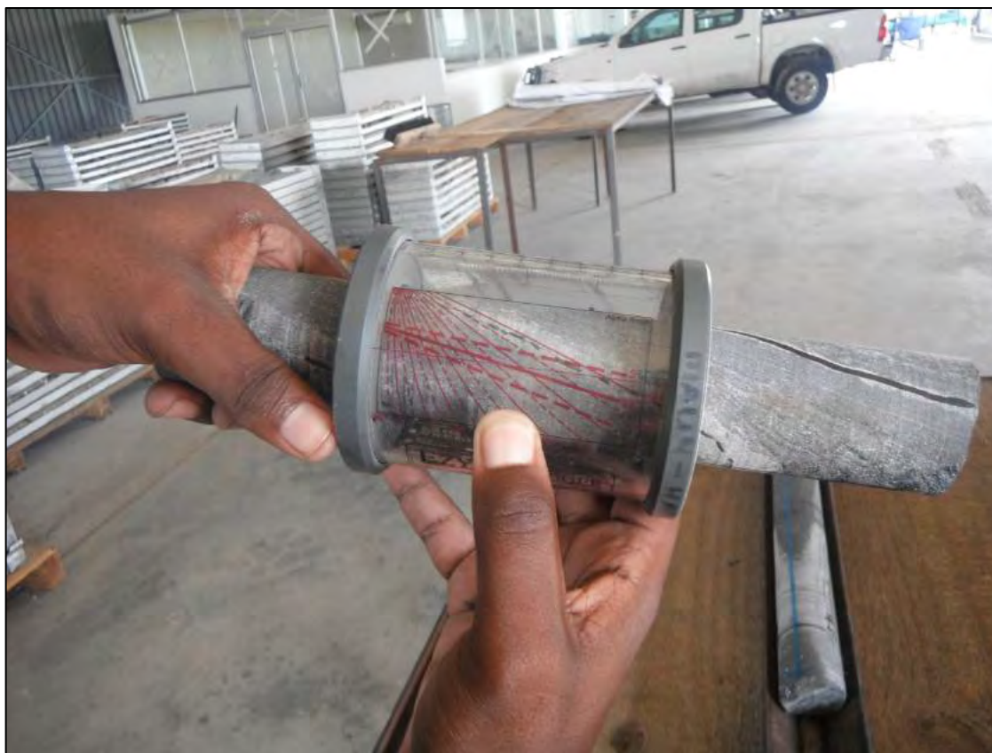
Figure 10-1: Structural core logging using EZY-Logger Goniometer (Source: SRK site visit, 2014)
