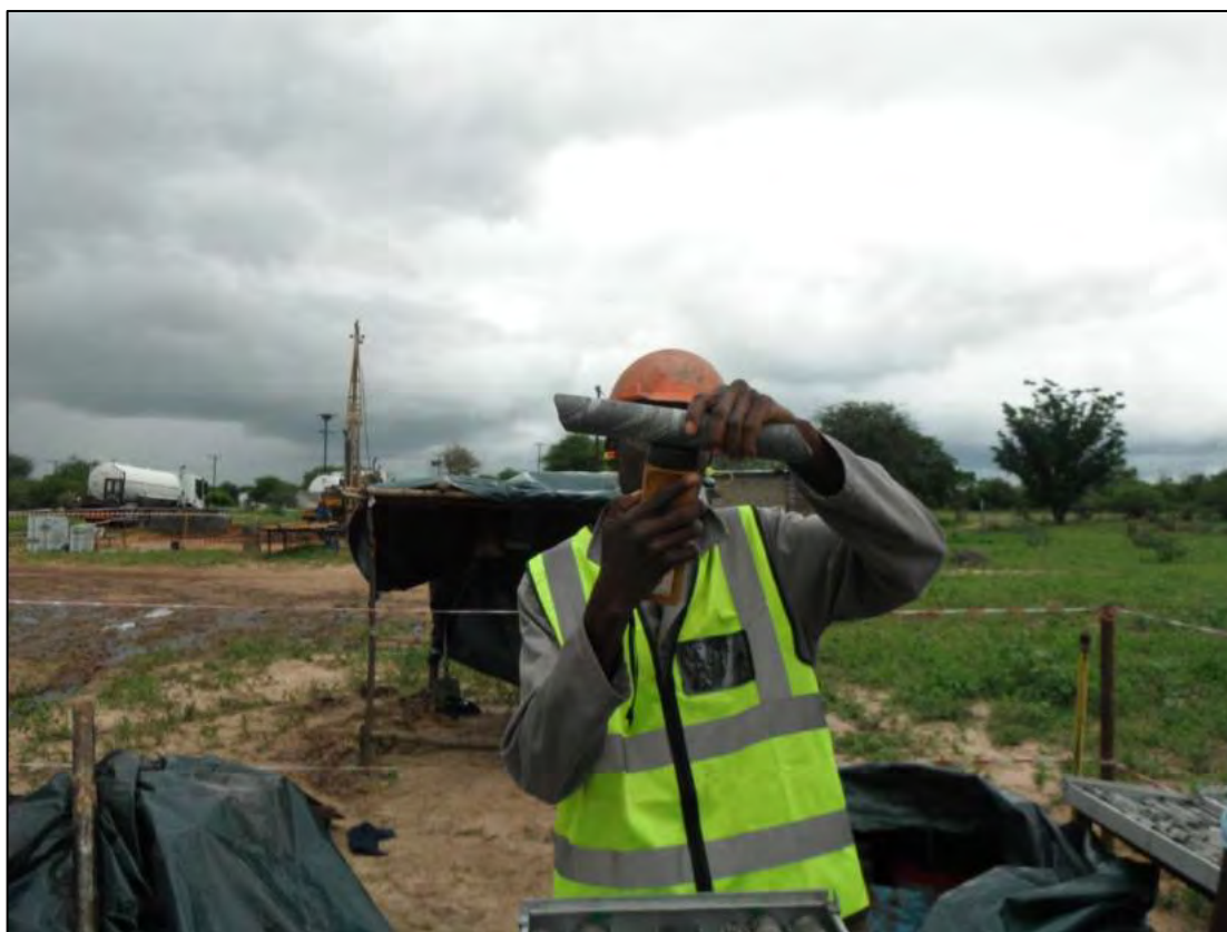
Figure 10-2: Magnetic susceptibility measurement at the drill rig (SRK site visit, 2014)
